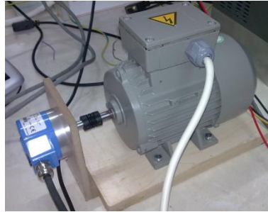
Fig. 4 Encoder and Asynchronous Motor
